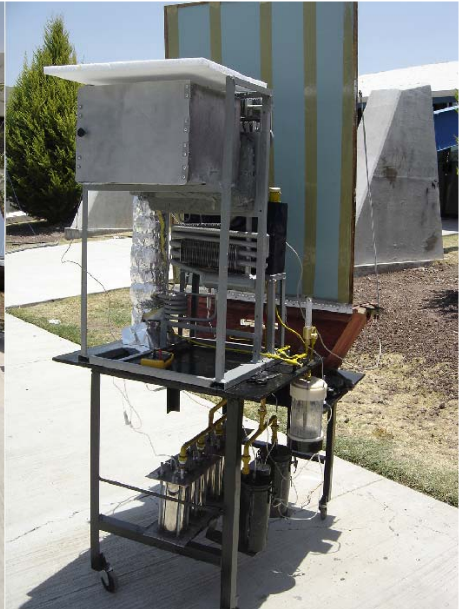
Tolokatsin 3 with solar refrigerator (photo to the right), and solar hot plate (photo to the left)
