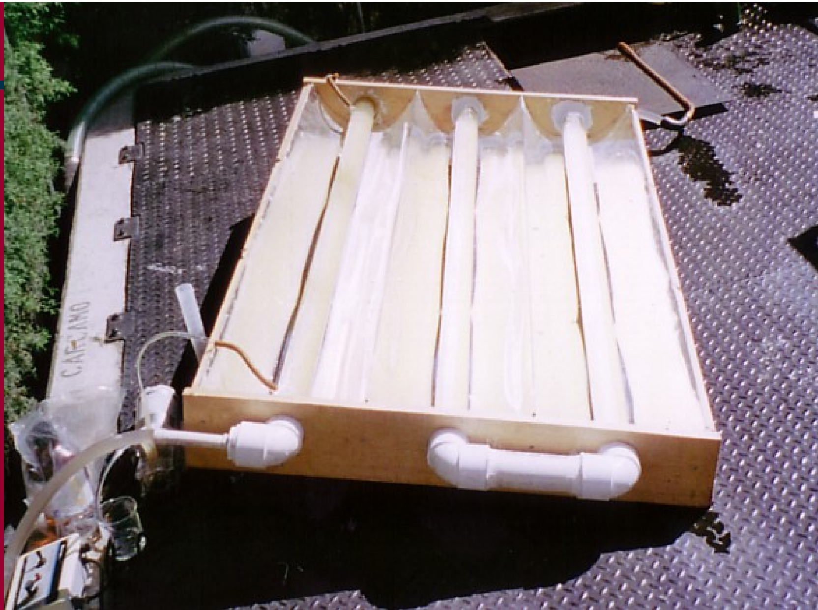
Home-made solar concentrator for R&D on treatment of industrial polluted water
